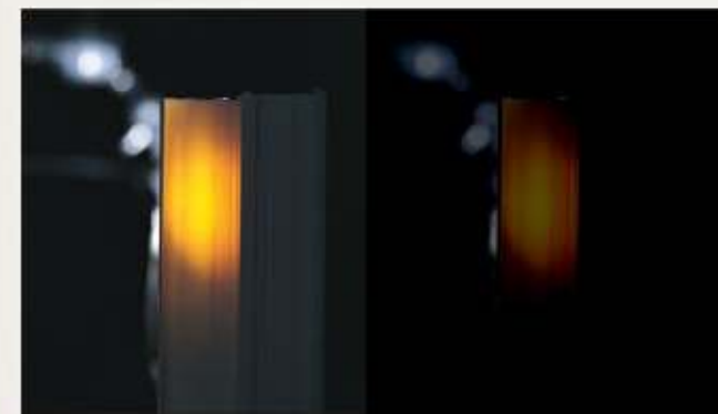
Light penetration of competitor's vinyl material
